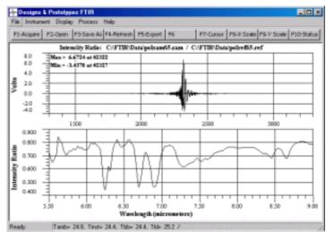
Display options enable the user to display interferograms, spectra or both, as well as to adjust plot scales and units. Onboard math processing allows for real-time calculation of ratio, difference, and absorbance, and when using our calibrated hot-cold blackbody calibrators, the ability to measure calibrated radiance.
