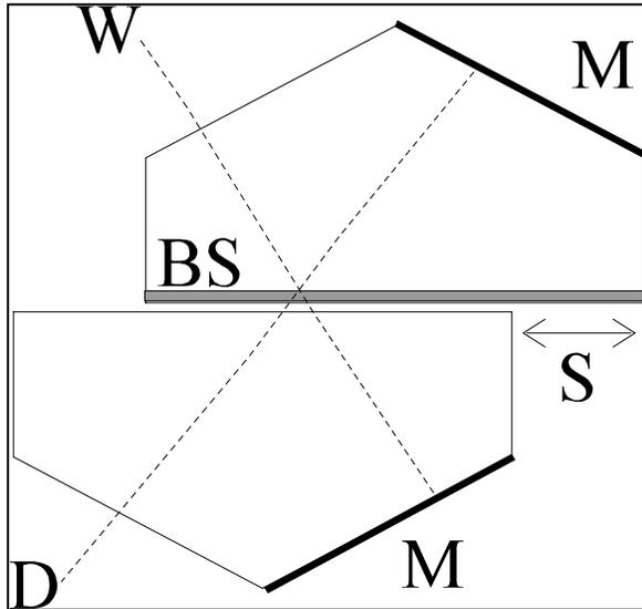
other half of the light passes through BS, and enters the other prism. It is reflected by the mirror coating M on that prism, then recombines at BS with the other half of the light that was originally reflected off BS. This causes the interference, with half the light returning to the source W, and half passing on to detector D. As the prisms scan back and forth, the path within one prism gets shorter and the path in the opposite prism gets longer, due to the angle of the two mirrors.
