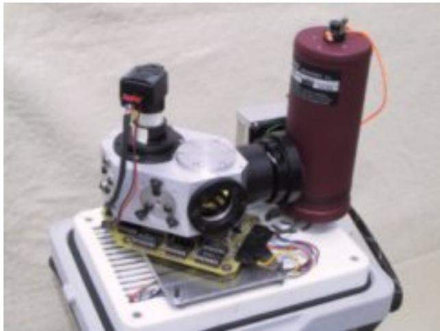
Figure 7. 16 element sensor, cover and telescope off
