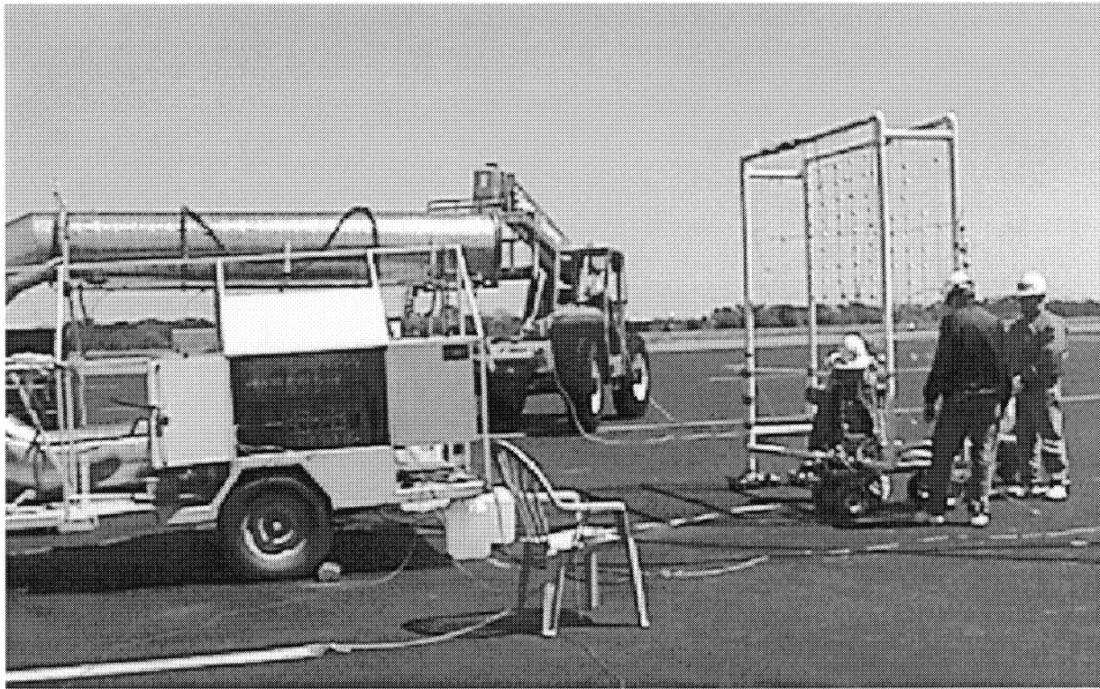
Figure 4. Waxahachie portable plume generator with horizontal stack configuration. Thermocouple array is on the right side of the figure.
